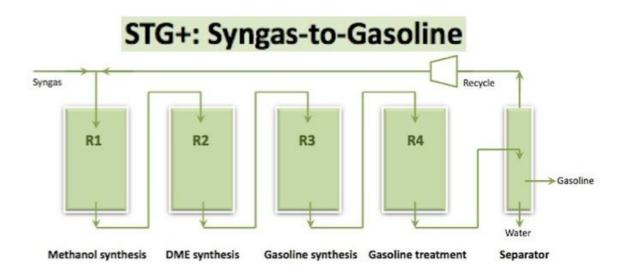
The STG+ process follows four principal steps in one continuous process loop. This process consists of four fixed bed reactors in series in which asyngas is converted to synthetic fuels. The steps for producing high-octane synthetic gasoline are as follows:
